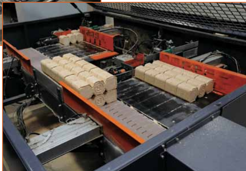
The wood briquettes are double stacked, fixed and wrapped with shrinking foil
