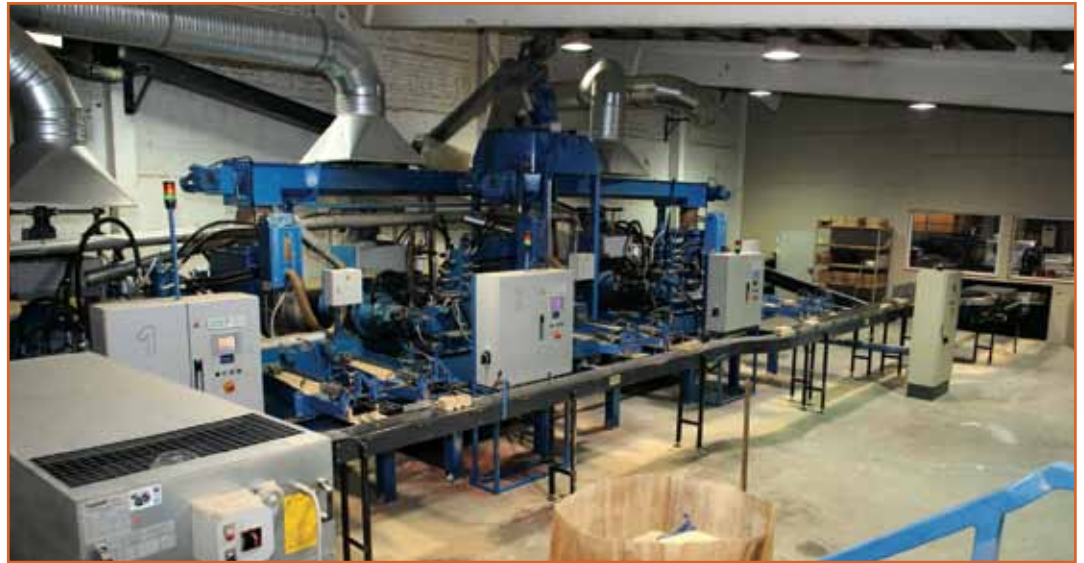
Robeta can produce roughly 3 tonnes of wood briquettes per hour on the three RUF briquetting presses which it currently owns. Space has already been planned for a possible fourth press
